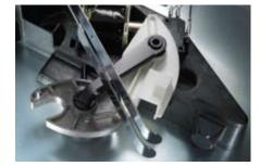
Heavy Duty Latch Mechanism
